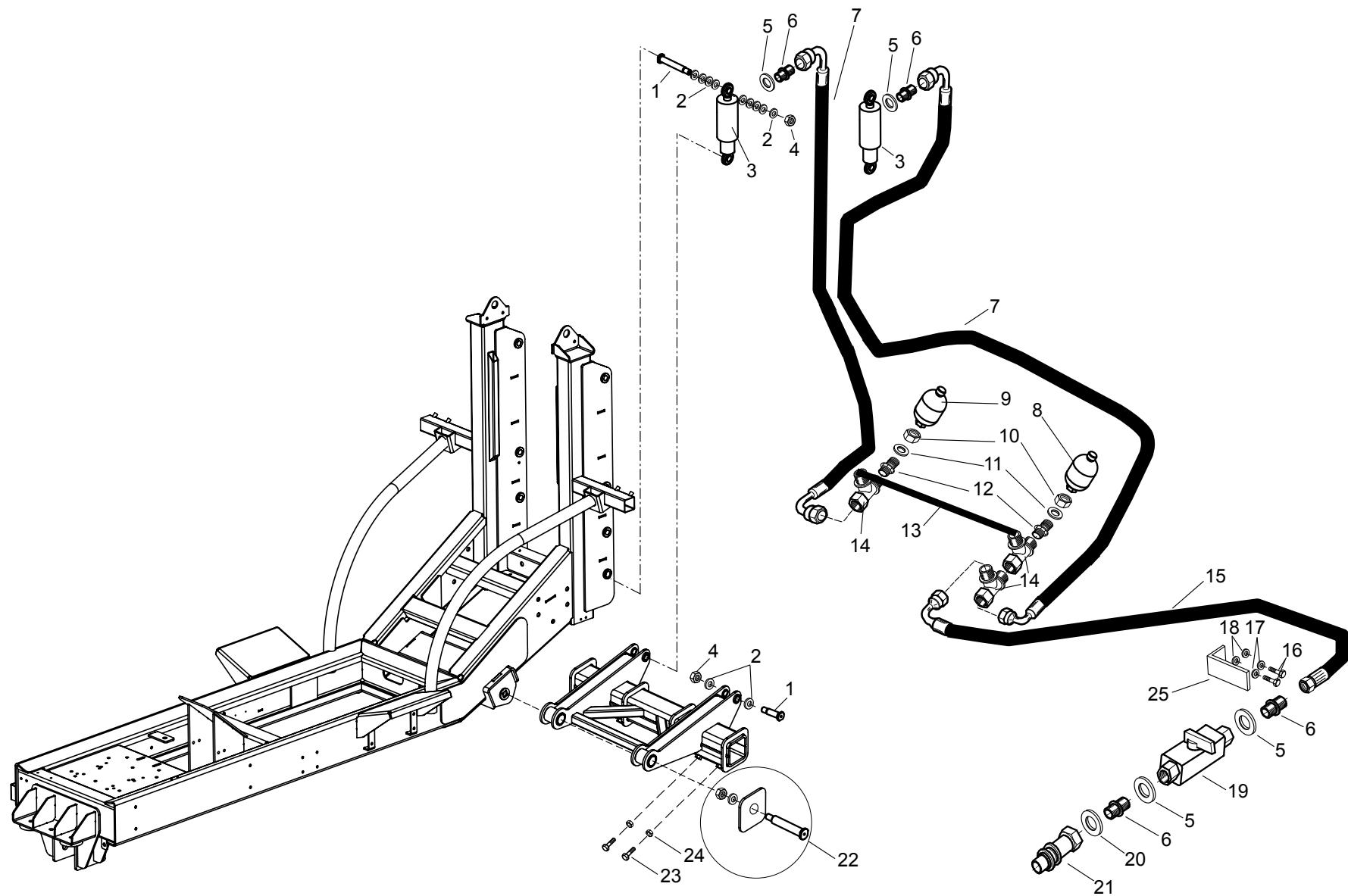
**Collegamenti sospensioni assale non sterzante / Non-steer axle connections suspension**
